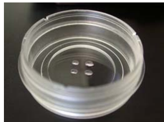
hydrophilic protein spots on hydrophobic, uncoated \mu -Dish
